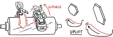
Let's take a closer look at the surface of an anilox and apply Newton's second law of rotation to a conventional anilox cell. As the anilox rotates, the ink inside each cell is pushed backwards colliding with the back-cell wall. This results in the ink rising from the cells creating a bubble effect on the surface of the anilox.
